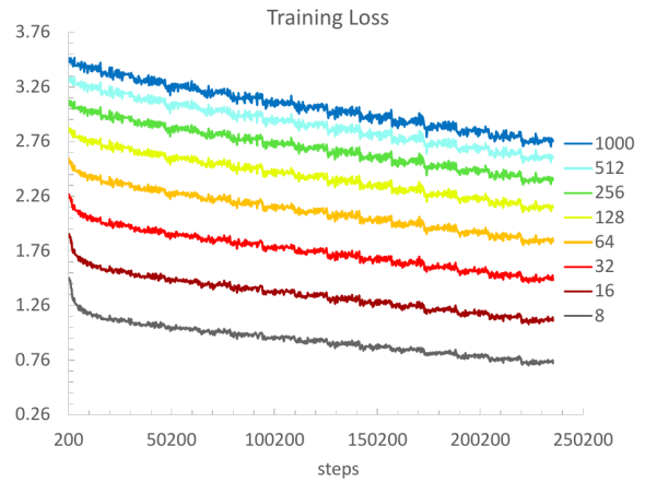
Figure 6: Evolution of the loss on the training set, as training of BM25→CODER(RepBERT) progresses. Different curves correspond to a different number of BM25 candidates used as negatives during training. While training loss is decreasing in all cases, only using a large number of candidates results in a significant improvement of performance over the base method on the validation and test sets (see Figure 2).
