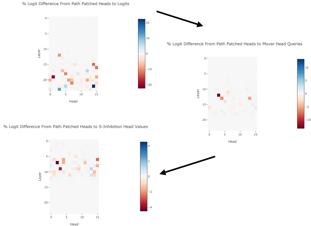
Figure 6: Full path patching results for the IOI task. Arrows show the three path patching iterations. Color bars show percent logit difference. The lower the number, the more important the head is, as patching it causes the logit difference to drop (i.e., harms performance). First the mover heads influence the logits. Path patching to the mover head query vectors (to see how these heads ‘decide’ where to attend) reveals the inhibition heads (12.3, 13.4, 13.14). Path patching to the value vectors of the inhibition heads (to see what the inhibition heads write into the residual stream), we find the induction and duplicate token heads, which are sensitive to the duplication of the subject token.
